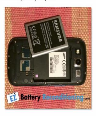
Step 3: Locate the polarity markings on your phone battery.
